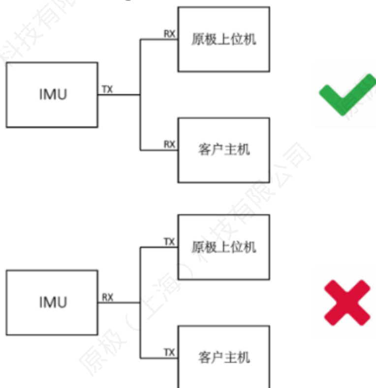
Figure 9 COM connection
